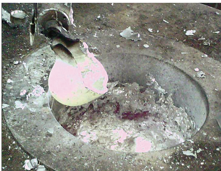
Opening in furnace because of using jaw
